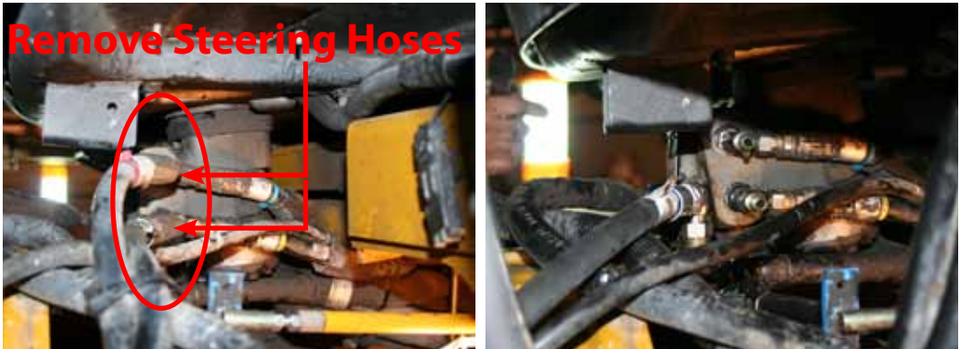
Figure 1-5: Removing Left and Right Steering Hoses
