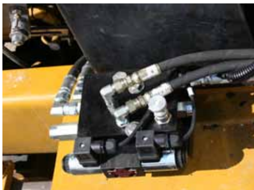
Figure 1-4: Mount FieldPilot Valve
